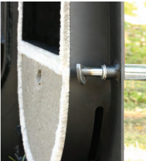
Special Canals inside the doors allows pre-heating combustion air via natural air flow.
