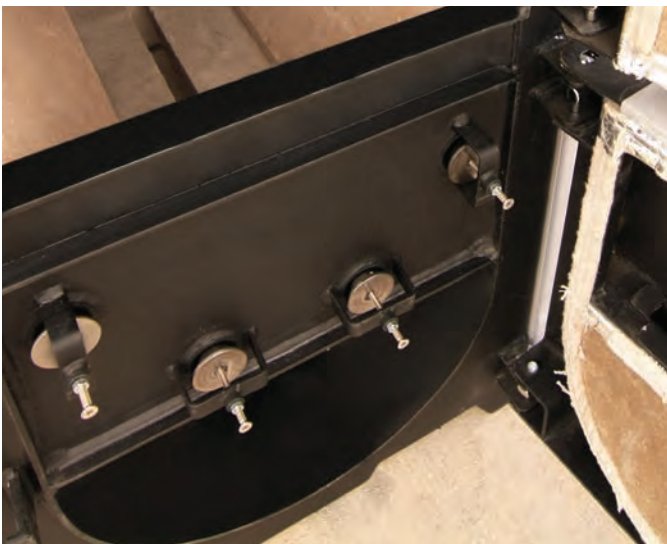
Independently adjustable Primary and secondary air inlets
